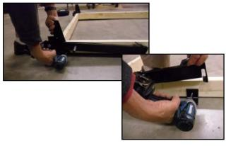
2. Fasten the front corner gussets at the front corners. These gussets are provided to add strength to the unit for lifting and moving.
