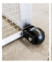
8. Bolt rear wheel assembly to back frame, lining up the bottom of the bracket with the bottom of the frame. (Wheels will extend slightly below the frame.) Carefully straighten wheel assembly before tightening nuts with 9/16" wrench or socket.
