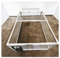
6. Fasten top frame to front half using four 3/8" X 1" hex bolts and nuts. Align sides and tighten bolts using 9/16" wrench and socket. (Not all sides may align perfectly.)
