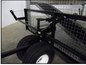
17.) Install the lift cylinder by pushing down on the tongue until the bolt lines up with the free end of the cylinder. Slide the cylinder onto the bolt and loosely secure it with a 5/16" lock nut.
