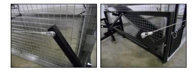
15.) Install the lift cable on the rear wheel assembly using  $5/16" \ge 11/2"$  carriage bolts and lock nuts. Then install the lift cables on the levers of the front lift frame using  $5/16" \ge 3/4"$  carriage bolts and lock nuts.
