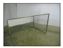
**2.)** Fasten the rear frame piece to the right end piece with two 3/8" x 1" bolts, one at the top and the other at the bottom. For now, only finger-tighten them.
