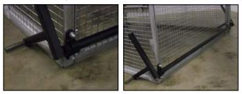
**14.)** Fasten the rear axle using two U-shaped brackets and four 3/8" x 1" bolts. Insert the bolts from the inside and secure the nuts on the outside to leave room for skirting.
