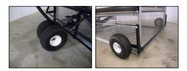
**16.)** Slide two wheels onto the front axle and secure with small cotter pins. Slide two wheels onto the rear axles and secure with small cotter pins.
