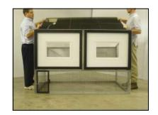
6.) With the help of another person, lower the floor, resting it on the angle iron tabs with the opening in the floor toward the back.
