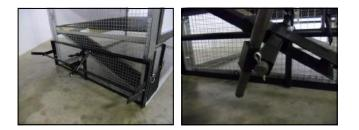
**13.)** Slide the lift frame under the left end of the Egg Cart'n and fasten it to the main frame with two 3/8" x 1" bolts, one at each end of the lift frame. Tighten the bolts securely (note: insert the bolts from the inside and secure the nuts on the outside to leave room for skirting). Slide the front wheel assembly onto the shaft of the lift frame and insert the large cotter pin below the axle.
