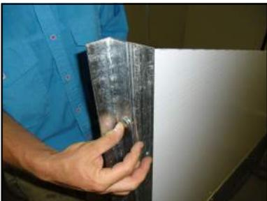
4.) Fasten the front piece to the ends with two carriage bolts on top and two hex bolts on bottom.
