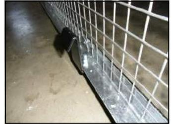
14.) Fasten the catches on the right and left sides with one 3/8" x 1" hex bolt.
