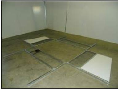
1.) Lay out the ends and sides of the Yolk Wagon with the angles of the frame face down.
