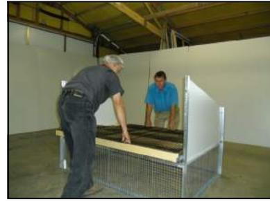
5.) Slide the floor into position between the end pieces, resting it on the support angles. When facing the unit, the front or tall side of the ladder and access hole should be on your left. Cut the plastic zip tie that holds the ladder in the up position for shipping.
