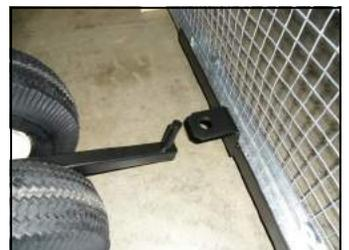
16.) Assemble the front-wheeled lift lever by sliding the wheels onto the axles and securing them with cotter pins. Insert the pin into the hole on the front lift bracket.
