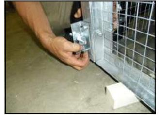
13.) Install the rear lift levers on both the right and left sides using 3/8" x 1" hex bolts. The pedals are installed with the shoe grip on top.
