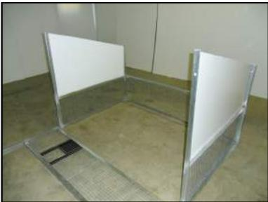
3.) Set up the left end, fastening it the same way, with one carriage bolt at the top and one hex bolt at the bottom.
