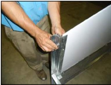
2.) Fasten the rear frame piece to the right end piece with a 3/8" x 1" carriage bolt at the top and a 3/8" x 1" hex bolt at the bottom. For now, only finger-tighten them.
